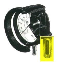
Internal Isolator. The 3D Internal Isolator GP400 prevents the passage of any contaminating product into the bourdon coil system, eliminating plugging. The unit is a sleeve-type elastomer which is threaded into the fitting of 3D gauges after liquid filling of the coil. The GP400 can be operated to full gauge pressure from -40' to + 250'F ( - 40'C to + 120' C) without deterioration of gauge accuracy, except on pressure ranges of 100 psi and under The GP400 is not suitable for gas service.
