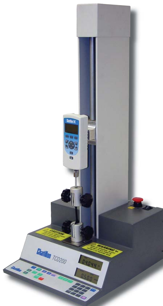
DFS Series force gauge shown with a TCD200 digital tester.
